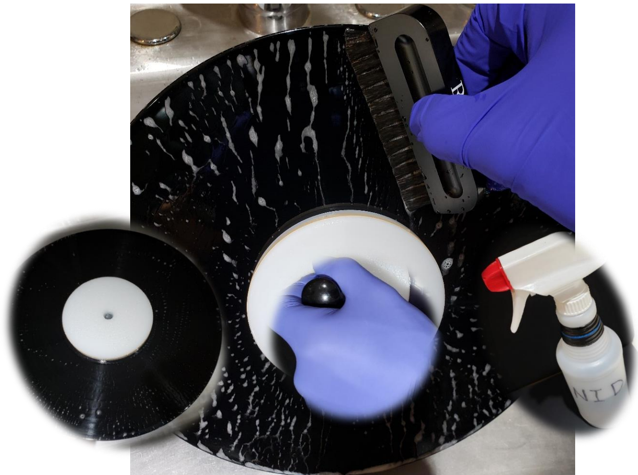
Figure 21 – Step 8: Final Clean with NID Solution & Brush
