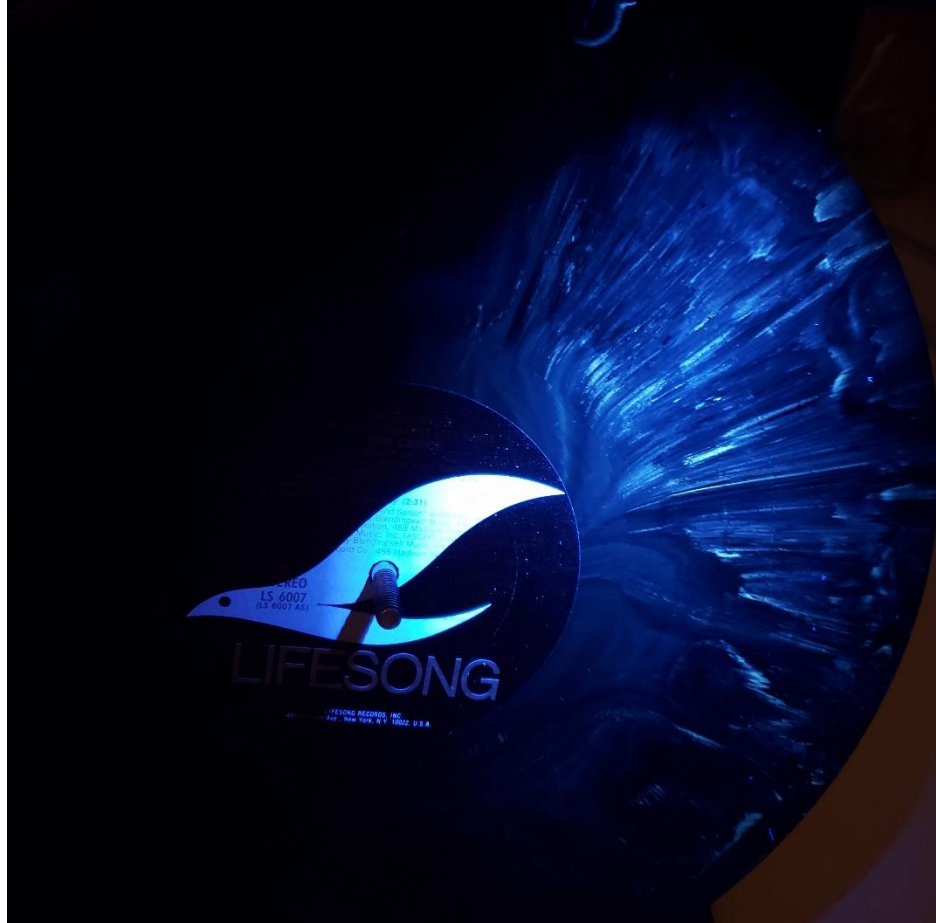
Figure 10 – Record Inspected UV Light – with Major Staining
