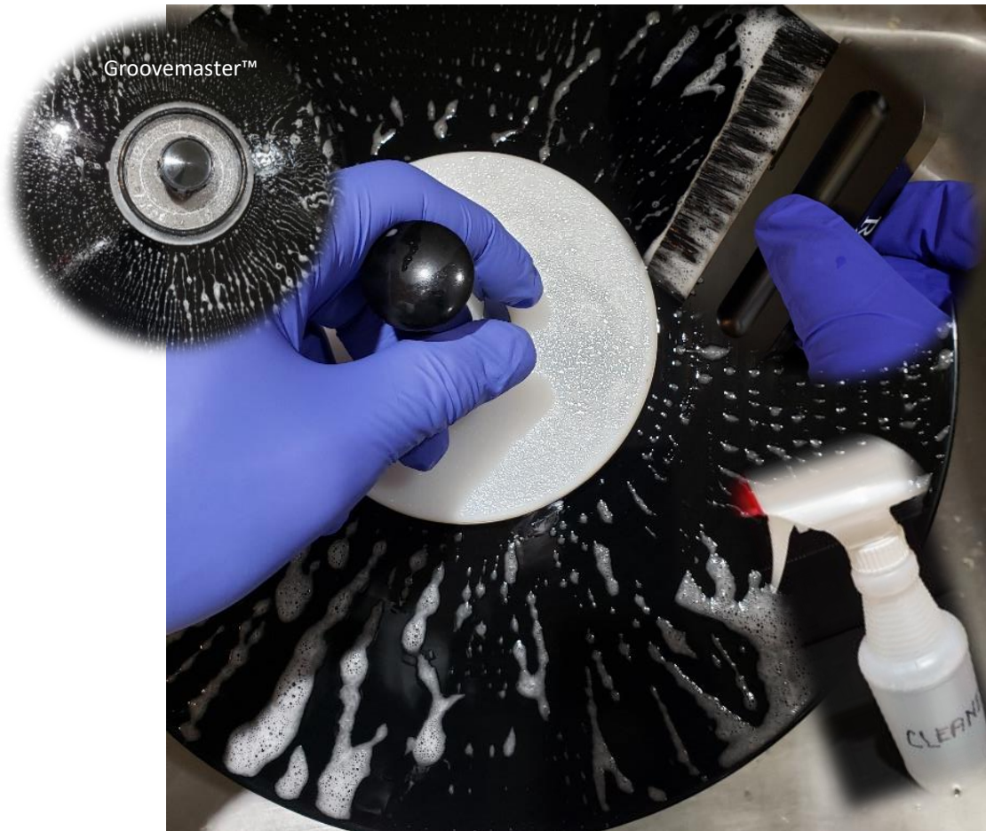
Figure 17 – Step 4: Pre-Clean with CLEANER Solution & Brush
