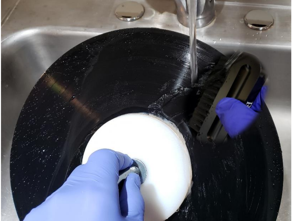
Figure 20 – Step 7: Acid Rinse with Tap Water & Brush
