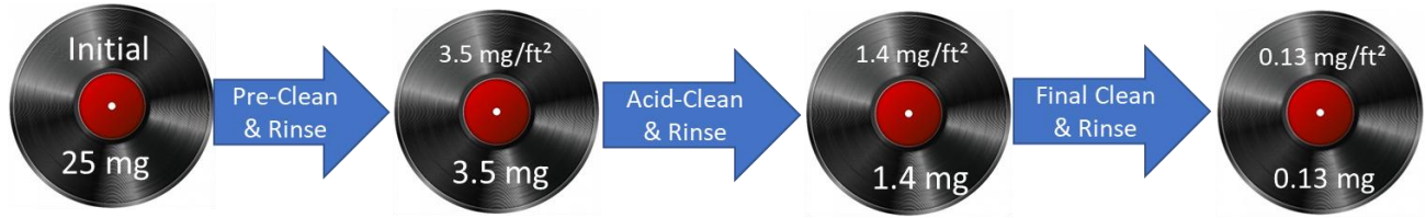
Figure 42 – Record NVR Following Precision Aqueous Cleaning Process
