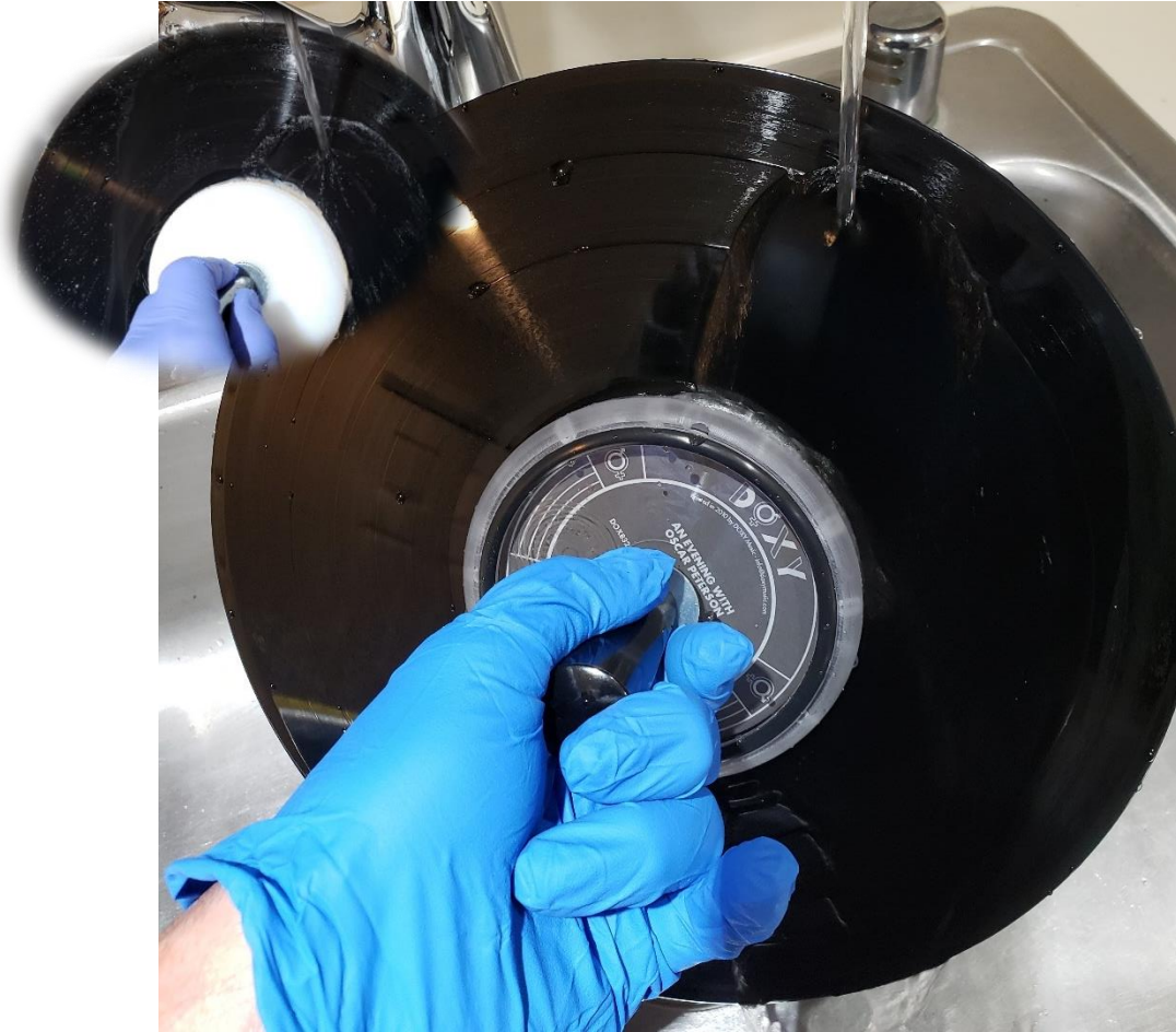
Figure 16 – Step 3: Pre-Rinse with Tap Water
