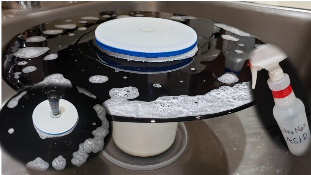
Figure 28 – Step 17: Record Acid Soak
