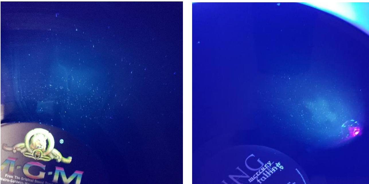
Figure 8 – Two New Records Inspected UV Light – Generally Clean
