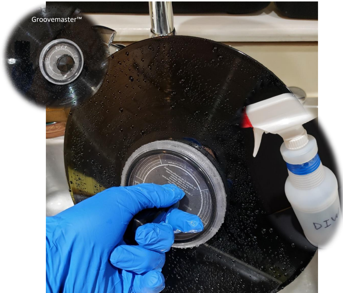
Figure 23 – Step 10: Final Spray Rinse with Distilled Water
