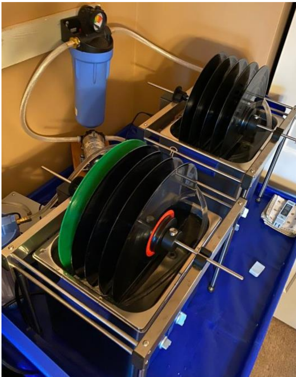
Figure 57 - Elmasonic™ UCM Filtered Clean/Rinse System & Kuzma™ RD Spinner w/Records
