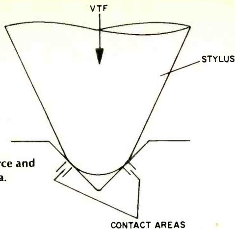
Fig. 3 — Vertical tracking force and contact area.
