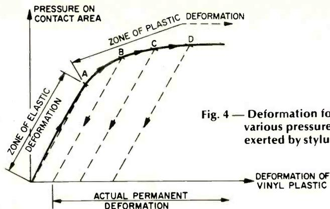
Fig. 4 — Deformation for various pressures exerted by stylus.
