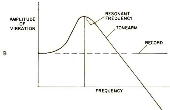
**Fig. 8 — A, deformation of a spring by adding mass; B, change in amplitude of vibration at resonant frequency.**
